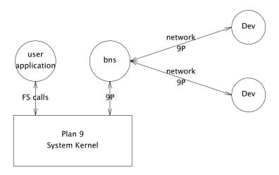
**Figure 1:** Bns provides resources by relying on external device file trees.
